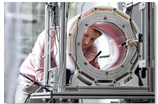
Figure 1: Image of the portable low-field MRI system in our laboratory. The scanner consists of hundreds of permanent neodymium magnets, arranged in a Halbach configuration to create the static 50 mT B_0 field.
