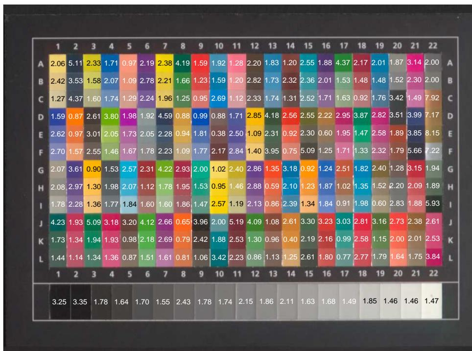
Figure 11: TE 221 test chart acquired with a flash light source and the corresponding  $\Delta E_{00}$  errors.
