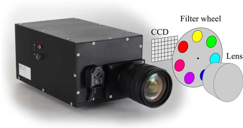
Figure 2: Our multispectral camera and a sketch of its internal configuration.
