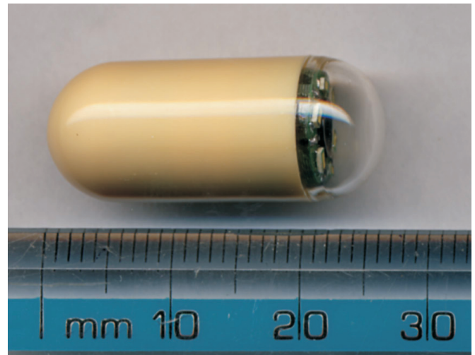
Fig. 4: Image of a capsule endoscope (pill-cam) with size reference
