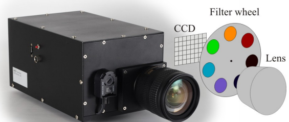
Fig. 1. Multispectral camera utilized at our institute. Seven optical bandpass filters in a filter wheel are placed between a monochrome sensor and a lens.
