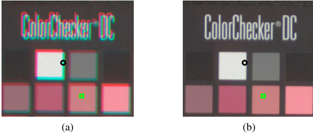
Fig. 9. Detail crop of RGB images, which have been reconstructed from unregistered (a) and registered (b) multispectral color components. The reconstructed spectra within the square and within the circle are shown in Fig. 10.
