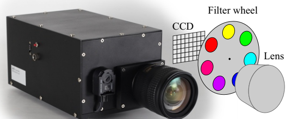
Fig. 1. Left: Our multispectral camera, using 7 optical bandpass filters. Right: Sketch of its internal configuration.
