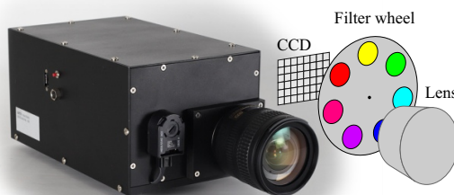
Figure 1. Our multispectral camera (left) and a sketch of its internal configuration (right).
