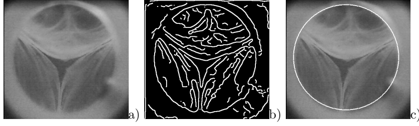
Figure 2. Original image (a), edge detection result (b) and Hough-segmented outline (c)
