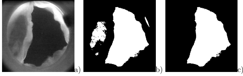
Figure 3. Valve image (a), thresholding result (b), and final result after center-based selection (c).
